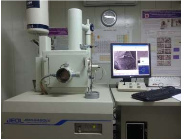
Resim 4.2. Tarama Elektron Mikroskobu (JEOL-JSM-6490LV Scanning Electron Microscope)
