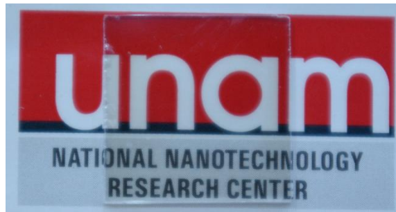
Figure 1.1: A quartz substrate with a 40-nm-thick ZnO film is placed over UNAM logo. The film is transparent under the visible light.
