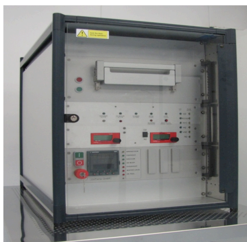
Figure 3.2: ATV-Unitherm (RTA SRO-704) rapid thermal annealing (RTA) system.
