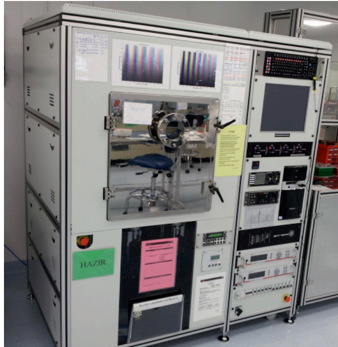
Figure 3.1: VAKSIS NanoD – 4S Magnetron Sputtering system which was used for SiO 2 , ZnO, Ti and Au thin film depositions.
