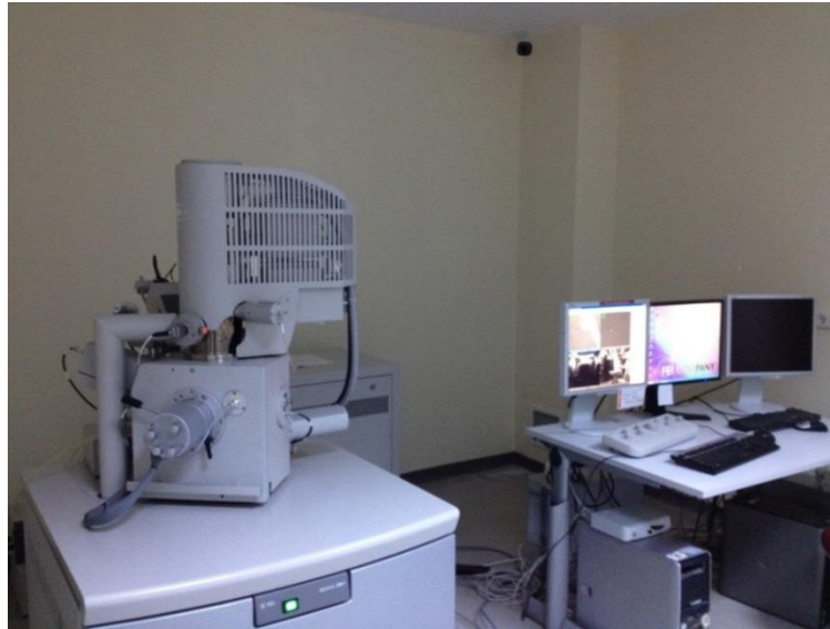
Figure 3.14 The scanning electron microscope used for the experiments presented here (FEI Quanta 200 FEG), available at the National Nanotechnology Research Center (UNAM).
