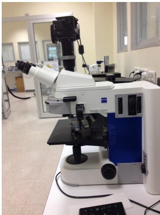
Figure 3.7 The optical microscope used for the work presented here (Carl Zeiss Axio Imager.A2m).
