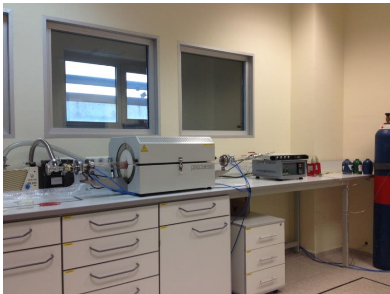
Figure 2.2 A picture of the CVD system at the National Nanotechnology Research Center (UNAM) used for the experiments reported in thesis.
