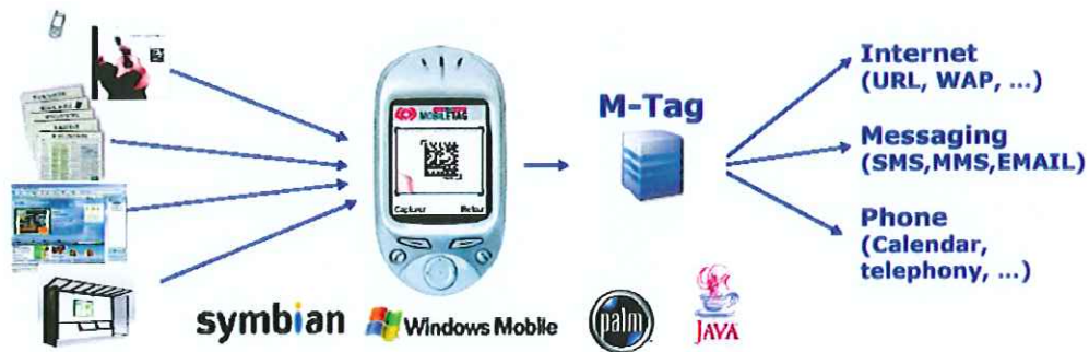
Figure14.7: How the Mobile Tag system works
