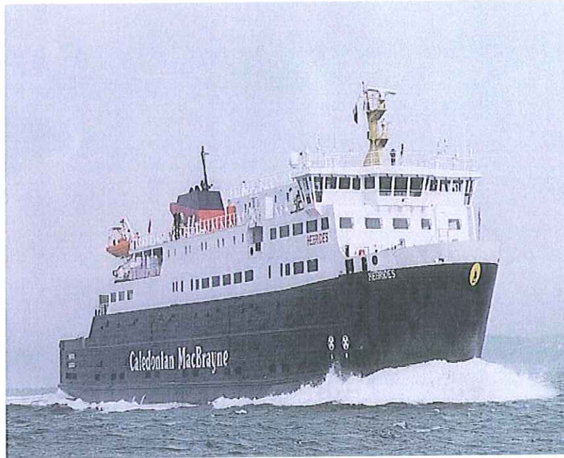
Figure 4.14 Twin Screw Ro-Ro passenger/car ferry
