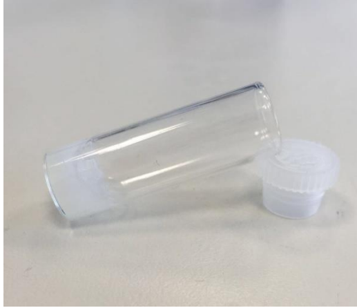
Figure 3.5 Mixing of positively and negatively charged PAs resulted in the formation of gels at pH 7.4.
