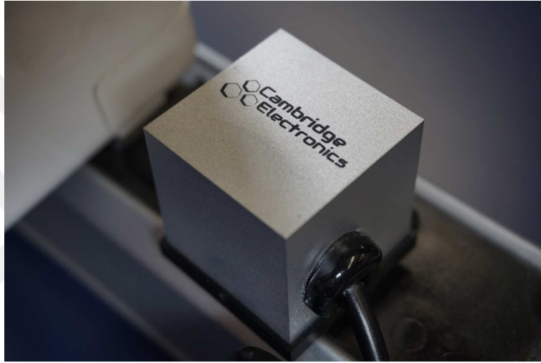
Figure 1.4: A prototype laptop power adapter made by Cambridge Electronics using GaN transistors. At 1.5 cubic inches in volume, this is the smallest laptop power adapter ever made.[4].
