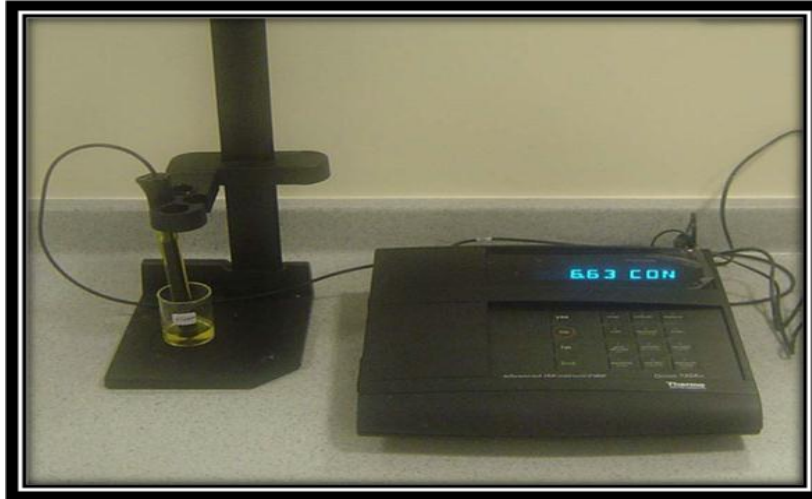
Resim 13: “Orion 720A+ ve Orion Fluorid Elektrodu (Thermo Orion Model 9609BN, combination fluide electrode with BNC connector)
