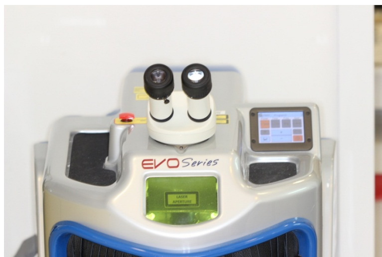
Figure3.8: Laser welding machine (Evo 100, Evo Series, Verona, Italy)
