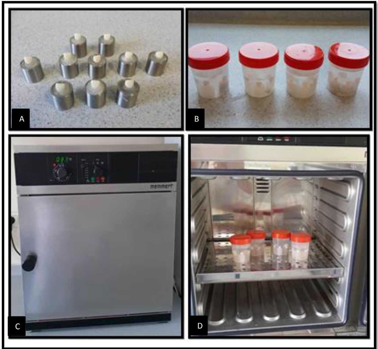
Figure 36. (A) Specimens (B) The Specimens were placed in distilled water (C) Incubator (Memmert GmbH + Co. KG) (D) Specimen were placed in the incubator
