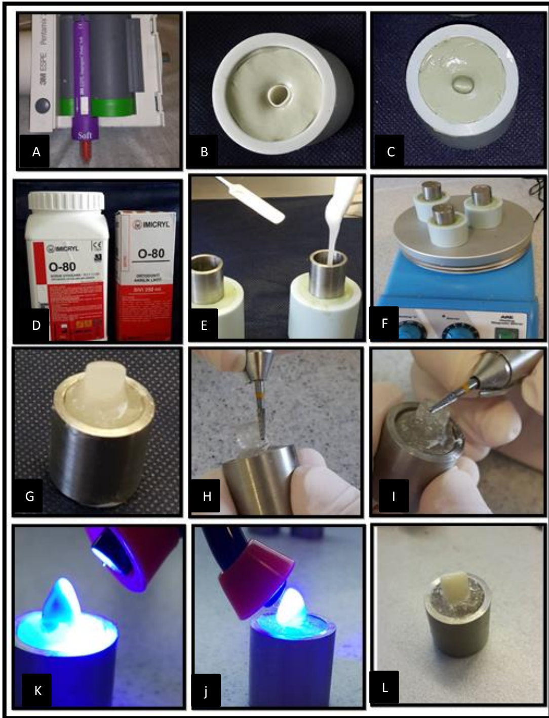
Figure 35. (A) Impregum Penta Soft; 3M ESPE, Seefeld, Germany (B,C) Negative replica of NuSmile® taken in the silicon mold (D) Imicryl 0-80 transparent self cure© Konya / TÜRKİYE ) (E) Pouring the acrylic die into the supporting metal (F) Specimens on dental vibrator (Vibrax Renfert USA) (G) Die specimen (H, I) Removal of undercut with an acrylic bur (K, J) Light cure the NuSmile® (L) Cemented specimen
