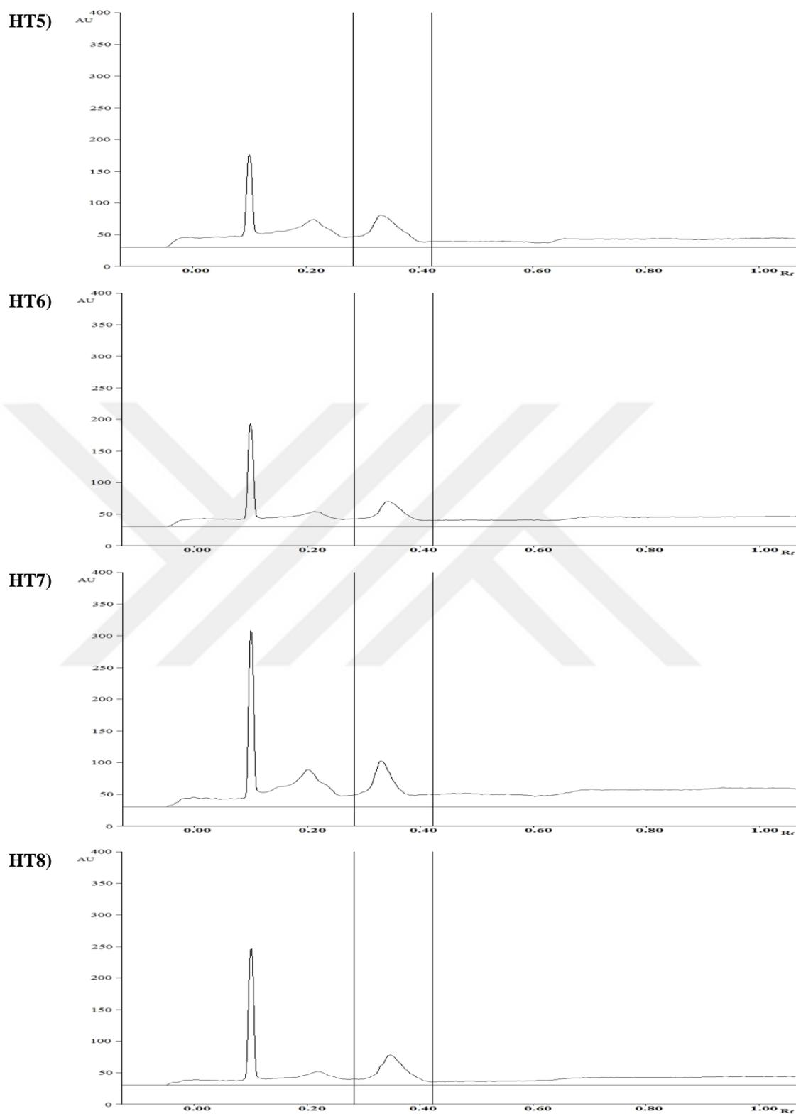
**Figure 4.29.** HPTLC densitograms from *H. perforatum* (SJW) tea products at 590 nm (continued). Test solutions of tea products: 40  $\mu\text{g}/\text{band}$ .
