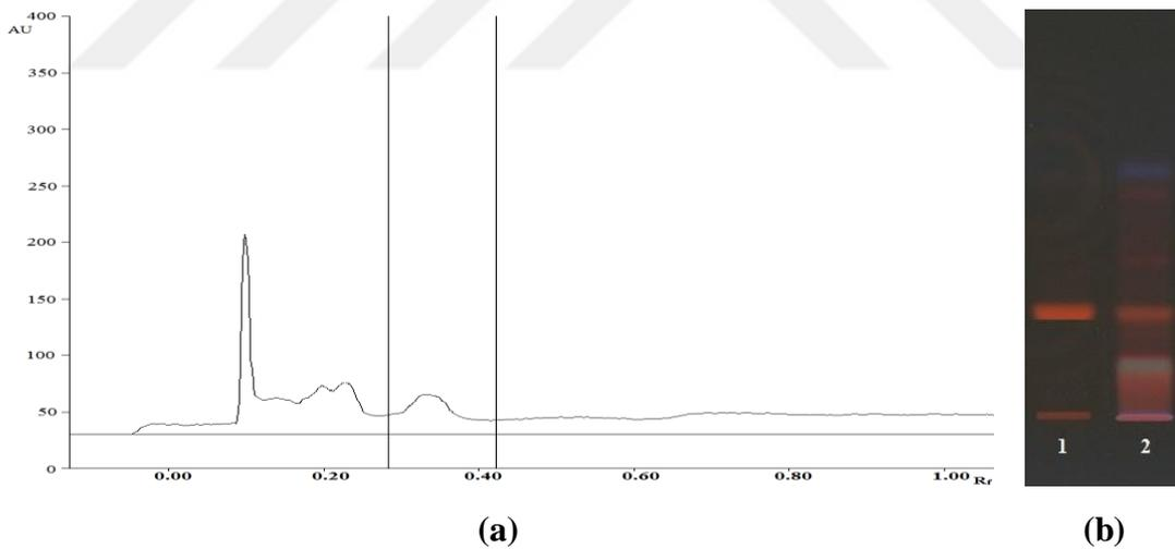
**Figure 4.31.** (a) HPTLC densitogram obtained from *H. perforatum* (SJW) capsule formulation at 590 nm (20  $\mu\text{g}/\text{band}$ ) and (b) HPTLC chromatogram of *H. perforatum* (SJW) capsule formulation at 366 nm. Tracks: (1) HyP reference (20 ng/band); (2) HC (20  $\mu\text{g}/\text{band}$ ).
