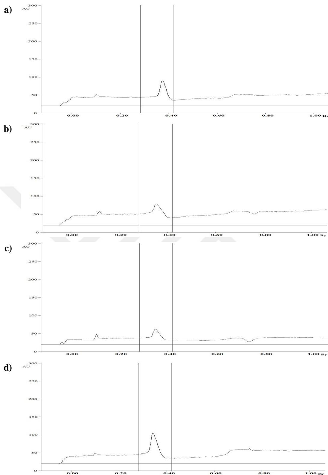
**Figure 4.35.** HPTLC densitograms obtained with the developed method for HyP at 590 nm extracted with various solvents from the oily preparation of *H. perforatum* (0.4 mg/band): (a) acetonitrile extract; (b) methanol-hexane extract; (c) acetone extract; (d) methanol extract.
