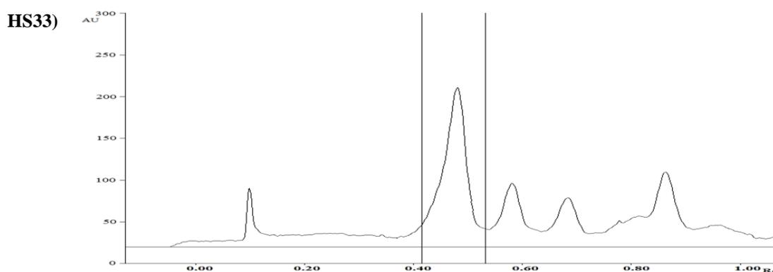
**Figure 4.50.** HPTLC densitograms from the marketed *H. perforatum* (SJW) herbal materials at 363 nm (continued). Sample test solutions: 10  $\mu\text{g}/\text{band}$ .
