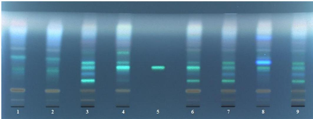
**Figure 4.48.** HPTLC chromatogram from *H. perforatum* (SJW) tea products at 366 nm. Tracks: (1) HT1; (2) HT2; (3) HT3; (4) HT4; (5) HyS reference (50 ng/band); (6) HT5; (7) HT6; (8) HT7; (9) HT8; applied volume of *H. perforatum* (SJW) tea products: 10  $\mu\text{g}$ /band; derivatization:  $\text{H}_2\text{SO}_4$  reagent.
