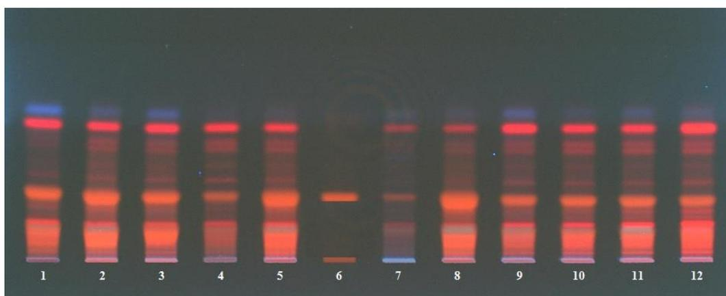
**Figure 4.33.** HPTLC chromatogram of the marketed *H. perforatum* (SJW) herbal materials at 366 nm (continued). Tracks: (1) HS12; (2) HS13; (3) HS14; (4) HS15; (5) HS16; (6) HyP reference (20 ng/band); (7) HS17; (8) HS18; (9) HS19; (10) HS20; (11) HS21; (12) HS22; applied volume of *H. perforatum* (SJW) herbal samples: 40  $\mu\text{g}/\text{band}$ .
