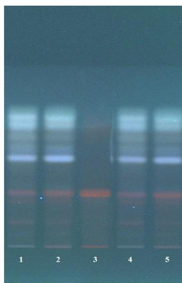
**Figure 4.36.** HPTLC chromatogram obtained with the developed method for HyP at 366 nm extracted with various solvents from the oily preparation of *H. perforatum*. Tracks: (1) acetonitrile extract; (2) methanol-hexane extract; (3) HyP (reference); (4) acetone extract; (5) methanol extract; derivatization: H<sub>2</sub>SO<sub>4</sub> reagent.
