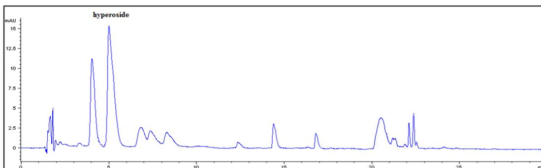
**Figure 4.40.** HPLC chromatogram of hyperoside in *H. perforatum* L. cultivar test solution at 360 nm
