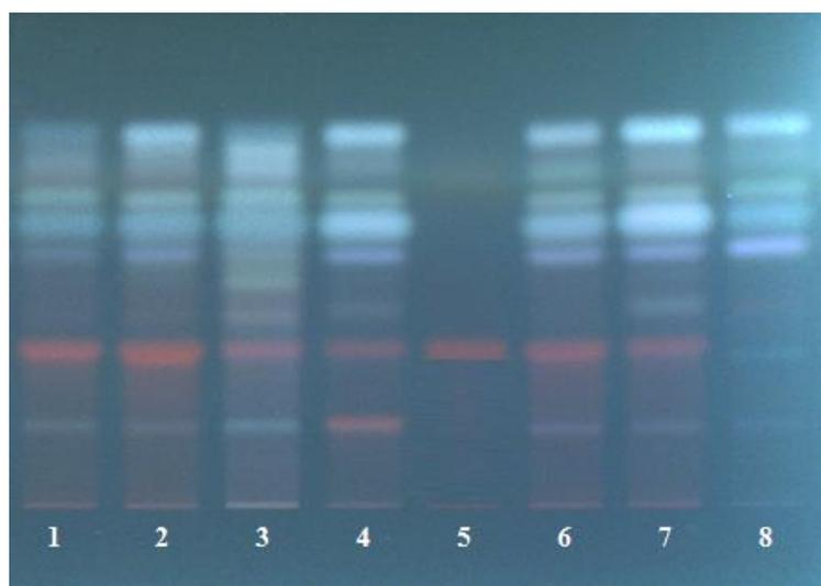
**Figure 4.38.** HPTLC chromatogram of the marketed *H. perforatum* (SJW) oily products at 366 nm. Tracks: (1) OE1; (2) OE2; (3) OE3; (4) OE4; (5) HyP (reference); (6) OE5; (7) OE6; (8) OE7; derivatization: H<sub>2</sub>SO<sub>4</sub> reagent.
