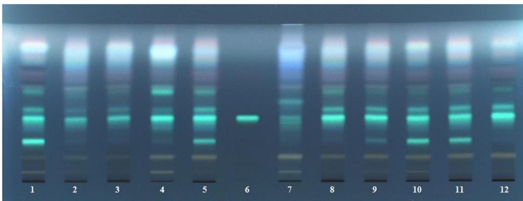
**Figure 4.51.** HPTLC chromatogram of the marketed *H. perforatum* (SJW) herbal materials at 366 nm (continued). Tracks: (1) HS12; (2) HS13; (3) HS14; (4) HS15; (5) HS16; (6) HyS reference (50 ng/band); (7) HS17; (8) HS18; (9) HS19; (10) HS20; (11) HS21; (12) HS22; applied volume of *H. perforatum* (SJW) herbal samples: 10  $\mu\text{g}$ /band; derivatization:  $\text{H}_2\text{SO}_4$  reagent.
