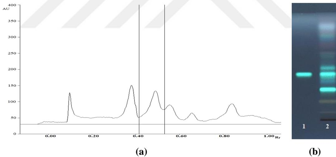
**Figure 4.49.** (a) HPTLC densitogram obtained from *H. perforatum* (SJW) capsule formulation at 363 nm (5  $\mu\text{g}$ /band) and (b) HPTLC chromatogram of *H. perforatum* (SJW) capsule formulation at 366 nm. Tracks: (1) HyS reference (50 ng/band); (2) HC (5  $\mu\text{g}$ /band); derivatization:  $\text{H}_2\text{SO}_4$  reagent.
