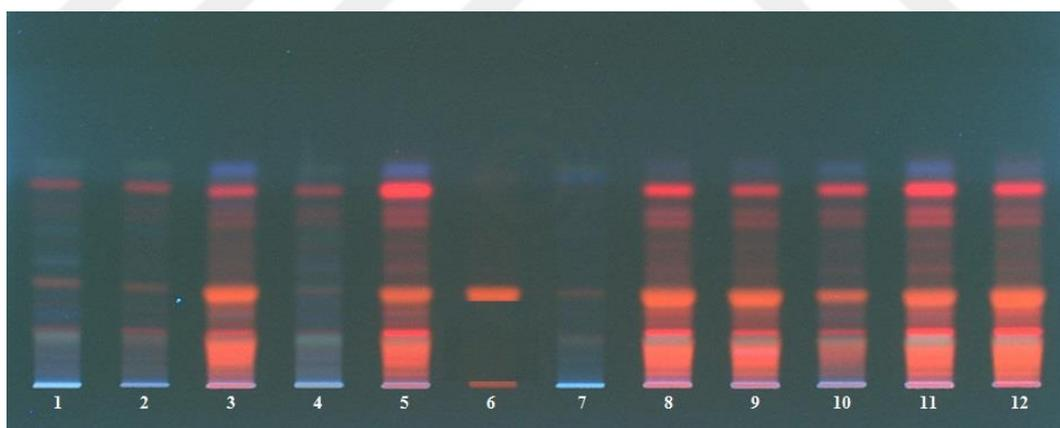
**Figure 4.33.** HPTLC chromatogram of the marketed *H. perforatum* (SJW) herbal materials at 366 nm (continued). Tracks: (1) HS23; (2) HS24; (3) HS25; (4) HS26; (5) HS27; (6) HyP reference (20 ng/band); (7) HS28; (8) HS29; (9) HS30; (10) HS31; (11) HS32; (12) HS33; applied volume of *H. perforatum* (SJW) herbal samples: 40  $\mu\text{g}/\text{band}$ .
