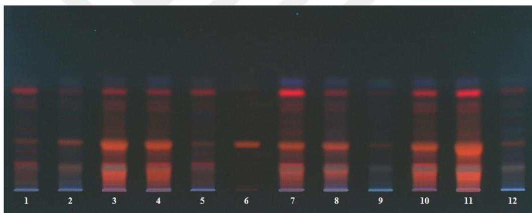
**Figure 4.33.** HPTLC chromatogram of the marketed *H. perforatum* (SJW) herbal materials at 366 nm. Tracks: (1) HS1; (2) HS2; (3) HS3; (4) HS4; (5) HS5; (6) HyP reference (20  $\text{ng}/\text{band}$ ); (7) HS6; (8) HS7; (9) HS8; (10) HS9; (11) HS10; (12) HS11; applied volume of *H. perforatum* (SJW) herbal samples: 40  $\mu\text{g}/\text{band}$ .
