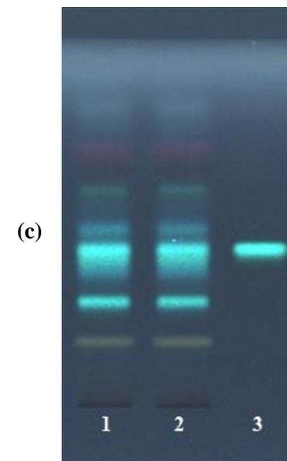
**Figure 4.52.** HPTLC densitograms obtained from the aqueous extracts of *H. perforatum* L. cultivar: (a) HP-W5 and (b) HP-W10 at 363 nm (10  $\mu\text{g}/\text{band}$ ); (c) HPTLC chromatogram of the aqueous extracts of *H. perforatum* L. cultivar at 366 nm.
