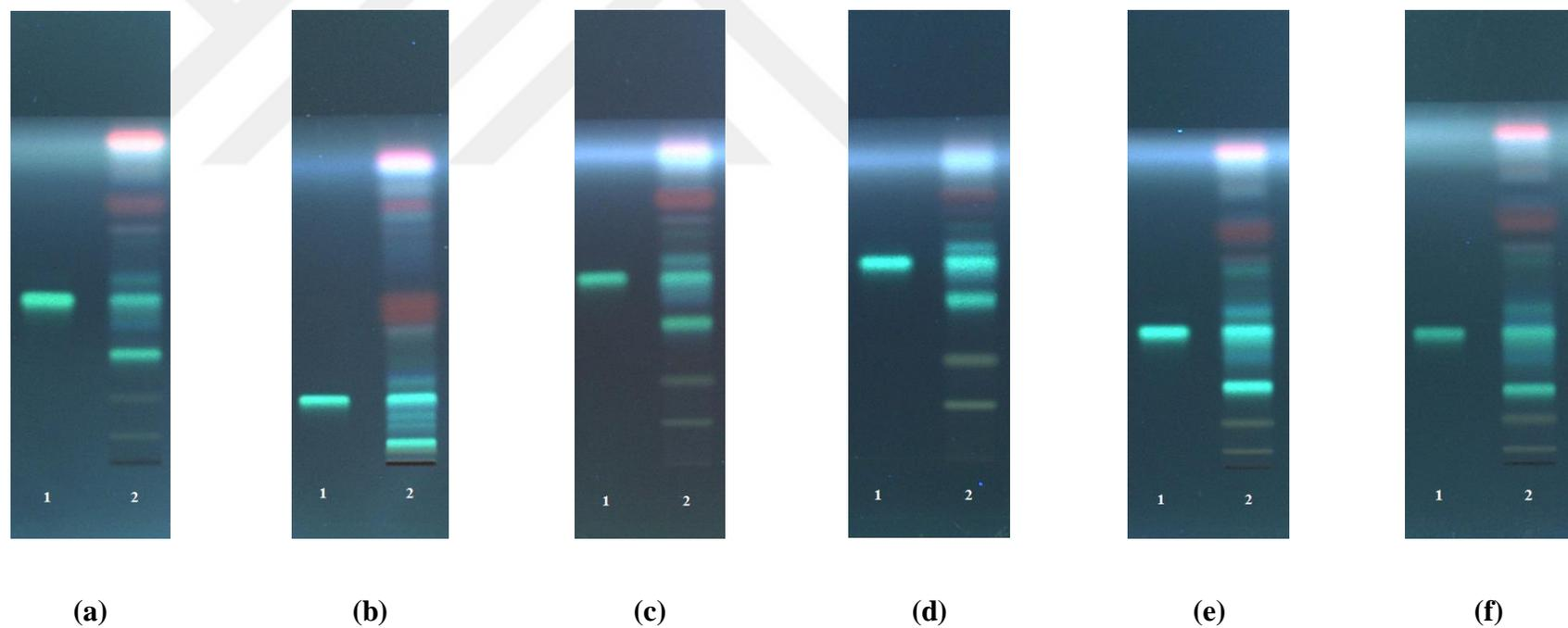
**Figure 4.42.** HPTLC chromatograms of HyS (reference) and the extract from the flowering aerial parts of *H. perforatum* L. cultivar obtained with various new mobile systems at 366 nm.
