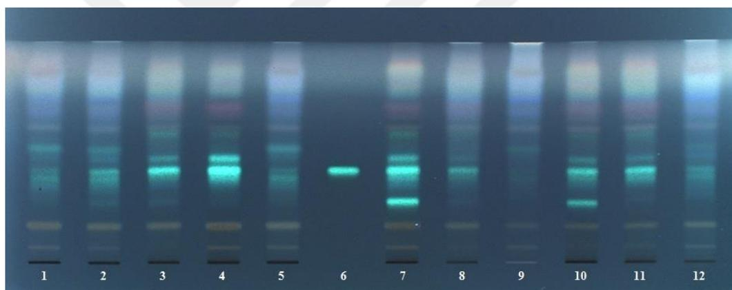
**Figure 4.51.** HPTLC chromatogram of the marketed *H. perforatum* (SJW) herbal materials at 366 nm. Tracks: (1) HS1; (2) HS2; (3) HS3; (4) HS4; (5) HS5; (6) HyS reference (50 ng/band); (7) HS6; (8) HS7; (9) HS8; (10) HS9; (11) HS10; (12) HS11; applied volume of *H. perforatum* (SJW) herbal samples: 10  $\mu\text{g}/\text{band}$ ; derivatization:  $\text{H}_2\text{SO}_4$  reagent.
