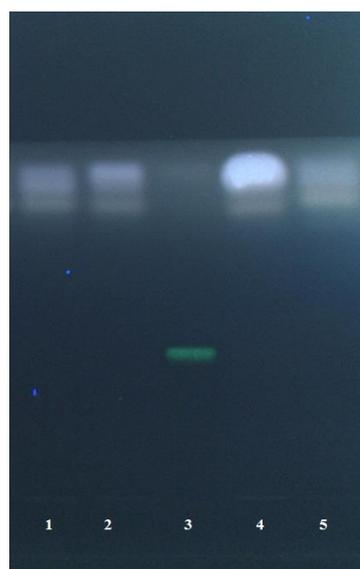
**Figure 4.53.** HPTLC chromatogram obtained with the developed method for HyS at 366 nm extracted with various solvents from the oily preparation of *H. perforatum*. Tracks: (1) acetonitrile extract; (2) methanol-hexane extract; (3) HyS (reference); (4) acetone extract; (5) methanol extract; derivatization: H<sub>2</sub>SO<sub>4</sub> reagent.
