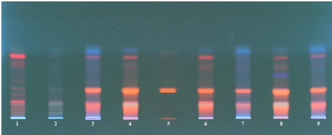
**Figure 4.30.** HPTLC chromatogram from *H. perforatum* (SJW) tea products at 366 nm. Tracks: (1) HT1; (2) HT2; (3) HT3; (4) HT4; (5) HyP reference (20 ng/band); (6) HT5; (7) HT6; (8) HT7; (9) HT8; applied volume of *H. perforatum* (SJW) tea products: 40  $\mu\text{g}/\text{band}$ .
