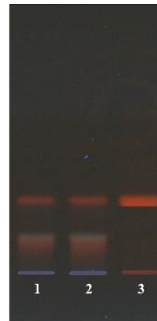
**Figure 4.34.** HPTLC densitograms obtained from the aqueous extracts of *H. perforatum* L. cultivar: (a) HP-W5 and (b) HP-W10 at 590 nm (40  $\mu\text{g}/\text{band}$ ); (c) HPTLC chromatogram of the aqueous extracts of *H. perforatum* L. cultivar at 366 nm. Tracks: (1) HP-W5 (40  $\mu\text{g}/\text{band}$ ); (2) HP-W10 (40  $\mu\text{g}/\text{band}$ ); (3) HyP reference (20 ng/band).
