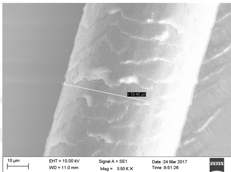
Figure 3.8. The image of natural blonde hair (diameter of hair strand is 59.46 \mu\text{m} ).
