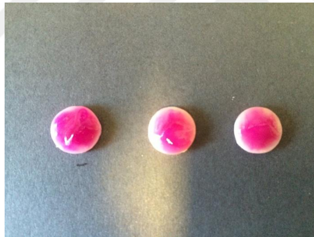
Figure 3.7: Application of the in-office bleaching material ( red gel ) on the top surface of 3 specimens
