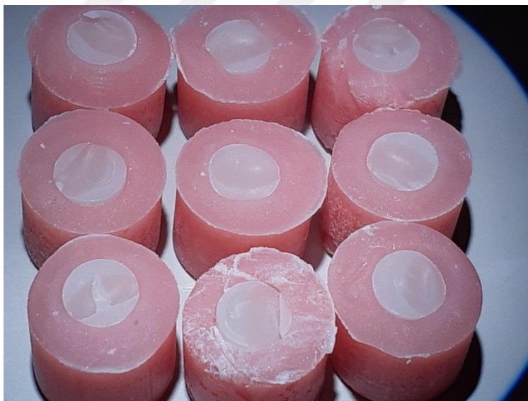
Figure 4.4: Cohesive failures among a number of the specimens.
