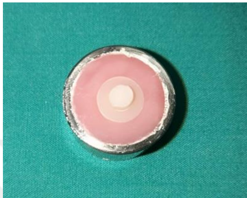
Figure 3.7: Specimen embedded in acrylic resin within a metal blocks.
