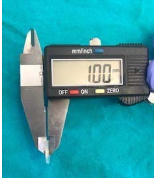
Figure 19. Measuring the thickness of dentin discs with digital calipers
