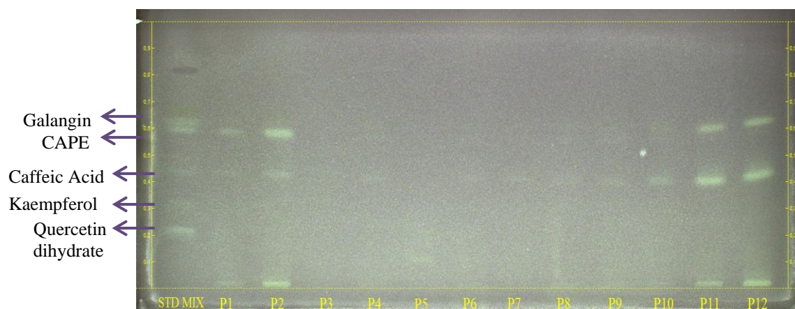
Figure 12. HPTLC- DPPH of P1-P12 propolis samples captured with white RT, developing solvent system n -hexane-ethyl acetate-glacial acetic acid (5:3:1 v/v/v), immersed in 0.1% DPPH solution
