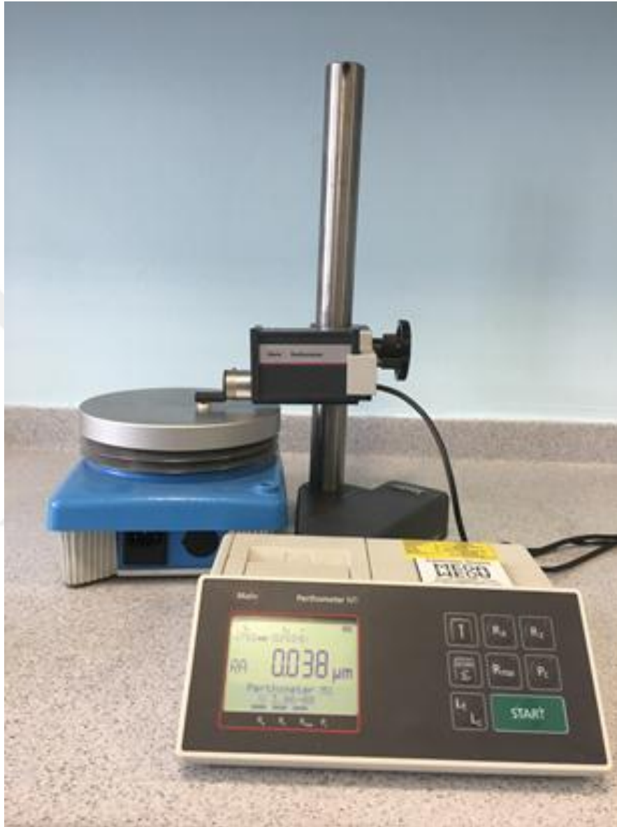
Figure 18: Perthometer MI device for surface roughness measurement
