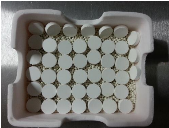
Figure 12: Pre-sintering zirconia disks with larger size
