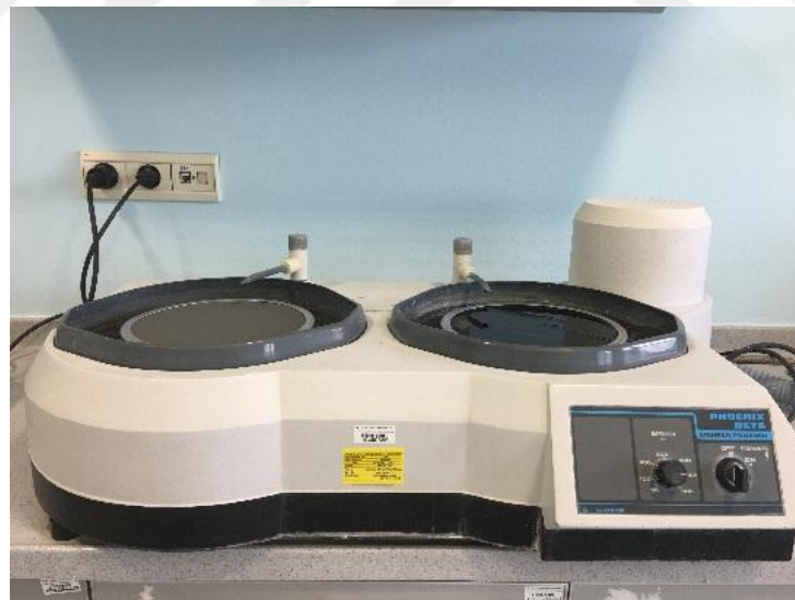
Figure 17: Polishing machine ( Phoenix Beta Grinder/ Polisher)
