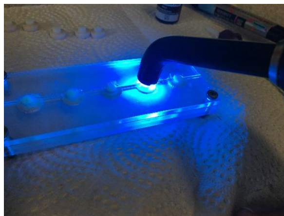
Figure 27: Light cure polymerization of the cement
