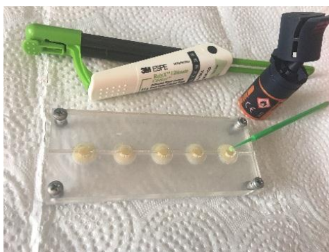
Figure 30: Primer applied by applicator brush
