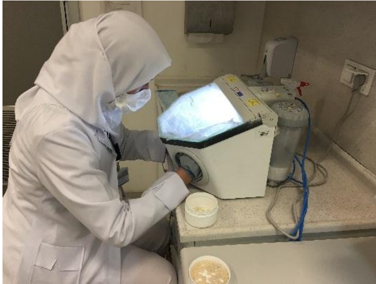
Figure 19: Airblasting with \text{Al}_2\text{O}_3 (Renfert, Basic master)
