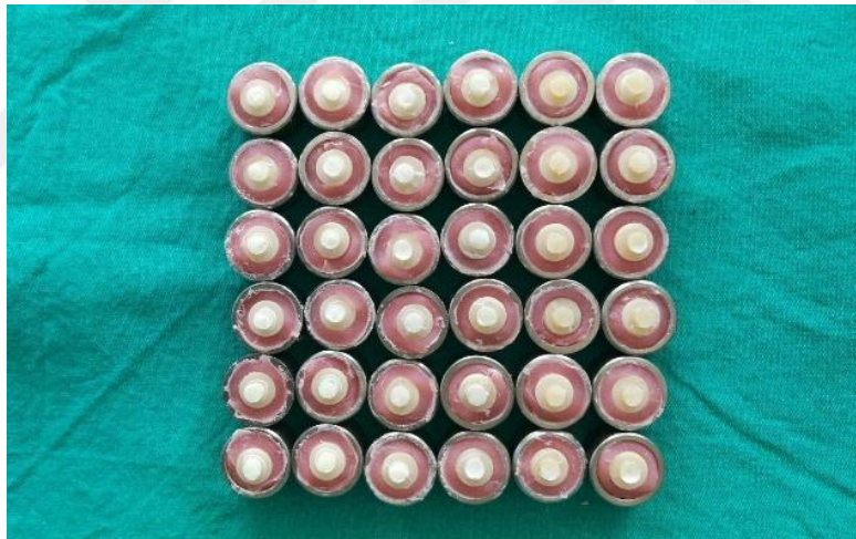
Figure 35: Samples embedded in a chemical acrylic resin
