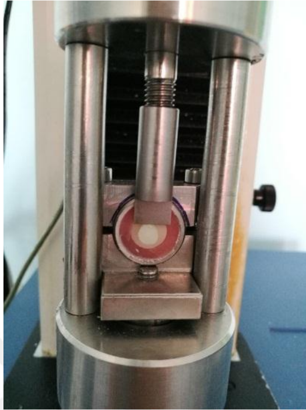
Figure 36: Samples fixed in the universal testing machine
