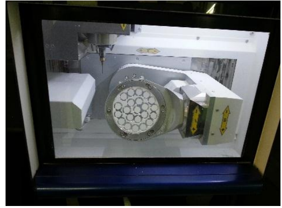
Figure 11: Milling of zirconia disks from presintered zirconium block
