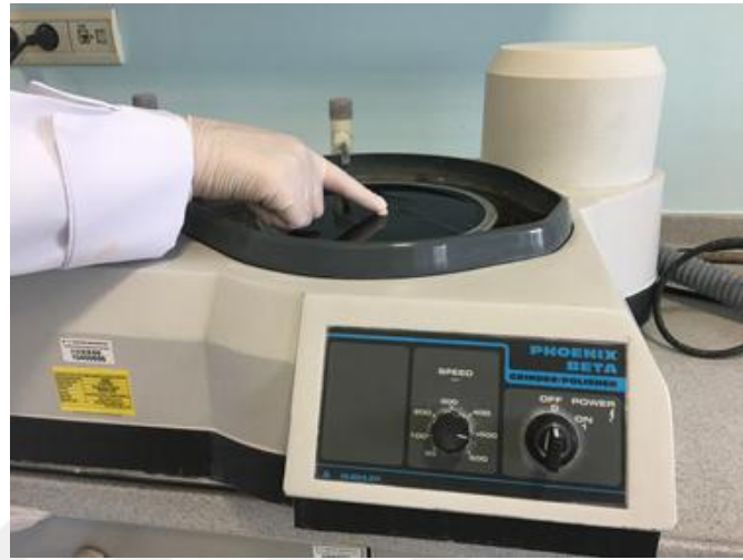
Figure 16: Polishing of zirconia bonding surface
