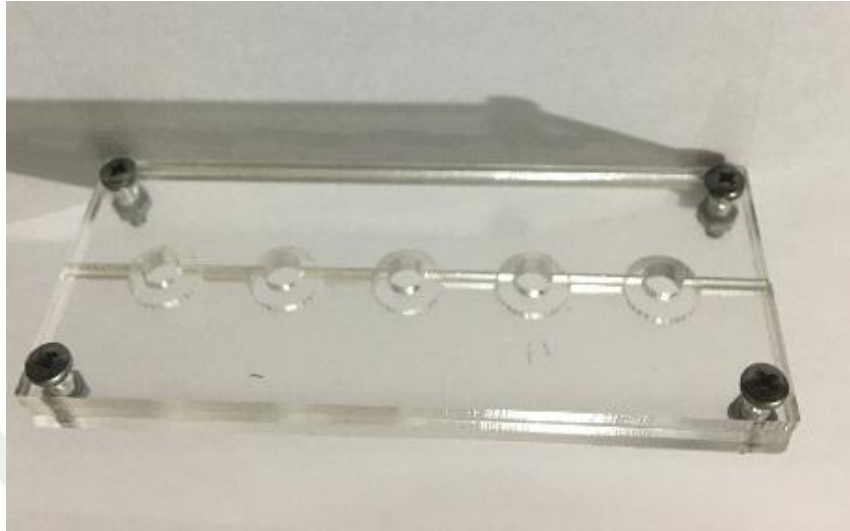
Figure 32: Translucent plastic split mold
