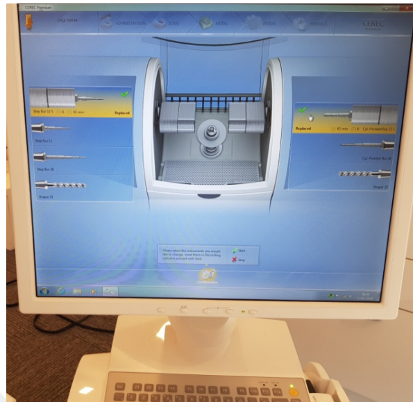
Figure 4: Display of the screen during refresh of the burs before using the device
