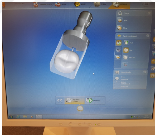
Figure 3: It is ready for production after the design of the crown. The buccal face of the remaining crown on the tij side is the lingual face of the crown close to the end of the block.
