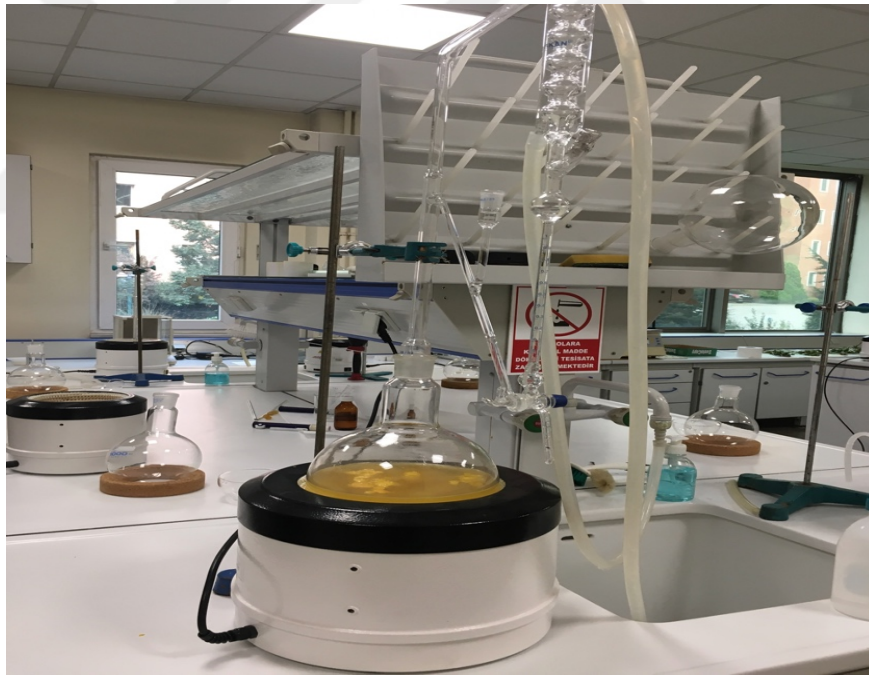
Figure 3.1. Distillation Set-up for Obtaining Citrus Sinensis Extract
