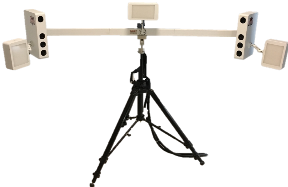
Figure 2.7.1. Stereophotogrammetry device with two camera pods and flashes.
