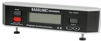
Figure.3.2: Baseline Digital Inclinometer
