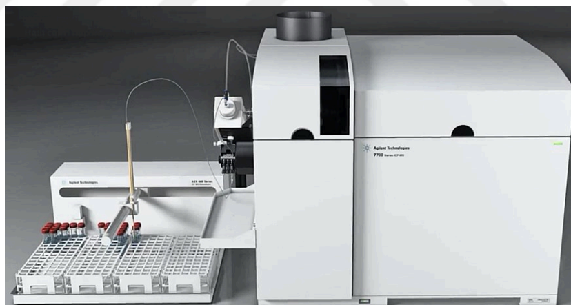
Fig. 3. 12. Released metal ions in the solutions were analyzed with ICP-MS. (163)
