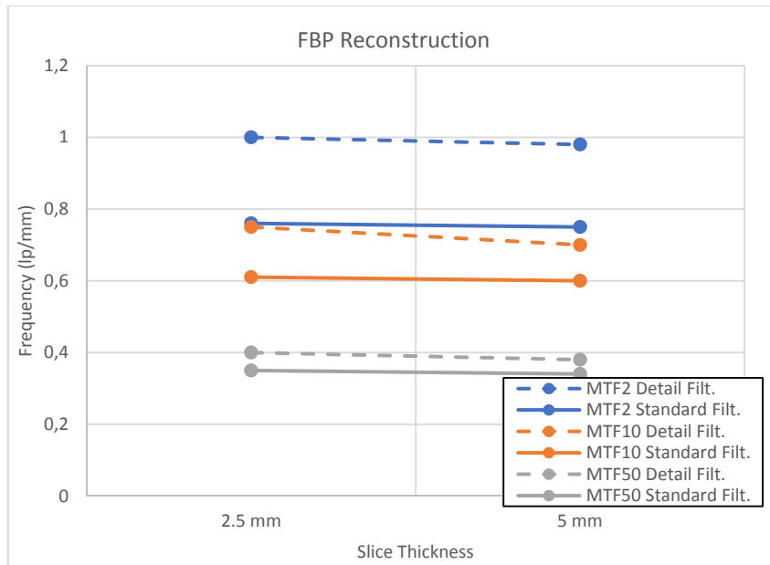
Figure A.5. MTF percentage values graphs for different slice thickness and reconstruction filters
