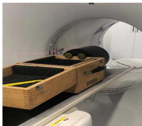
Figure 3.3. CT quality assurance phantom, Catphan 600, positioning to test
