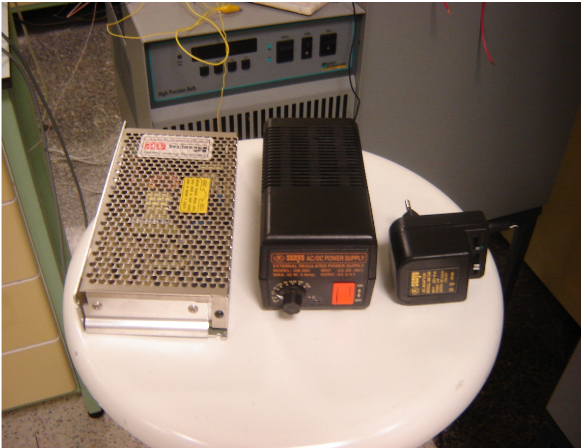
Figure 4.18 photograph of the power supplies from left to right 24V DC, 5V DC and 12V DC power supply
