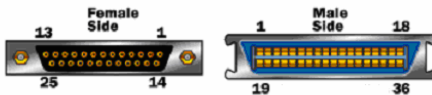
Figure 4.23 Female and male side of the parallel port
