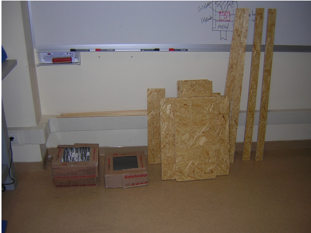
Fig.3.2.3.3.b: Main modeling materials as cut OSB board pieces and ceramic granite tiles
