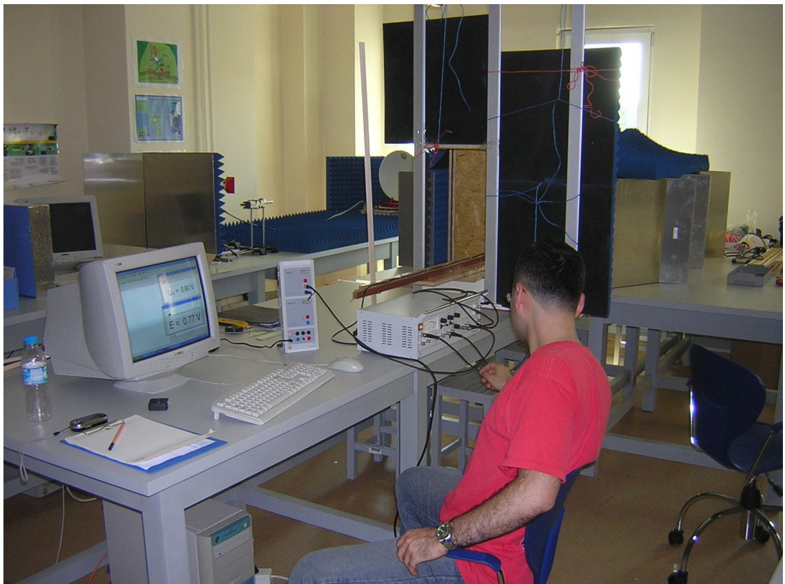
Fig. 3.2.3.3.k: Test equipment (from left to right desktop, the interface, and LD Power Supply&SWR meter)
