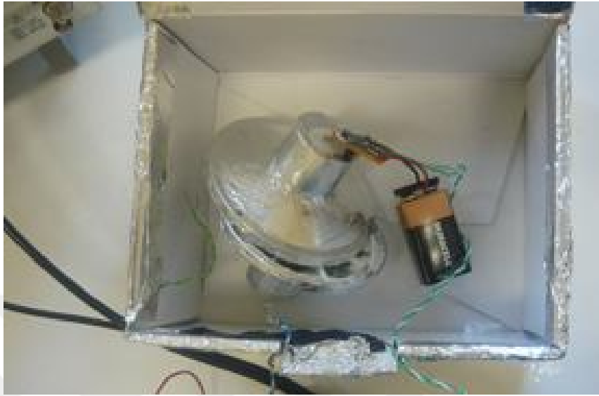
Figure 4.14. Receiver, printed circuit board and transmitter cones in the light isolation box
