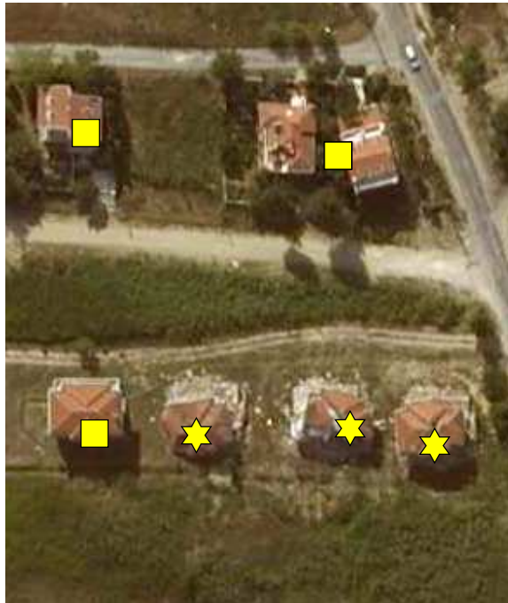
Figure 3.30. Detected buildings in Damage_2 test image. Detected damaged buildings are labeled with a star
