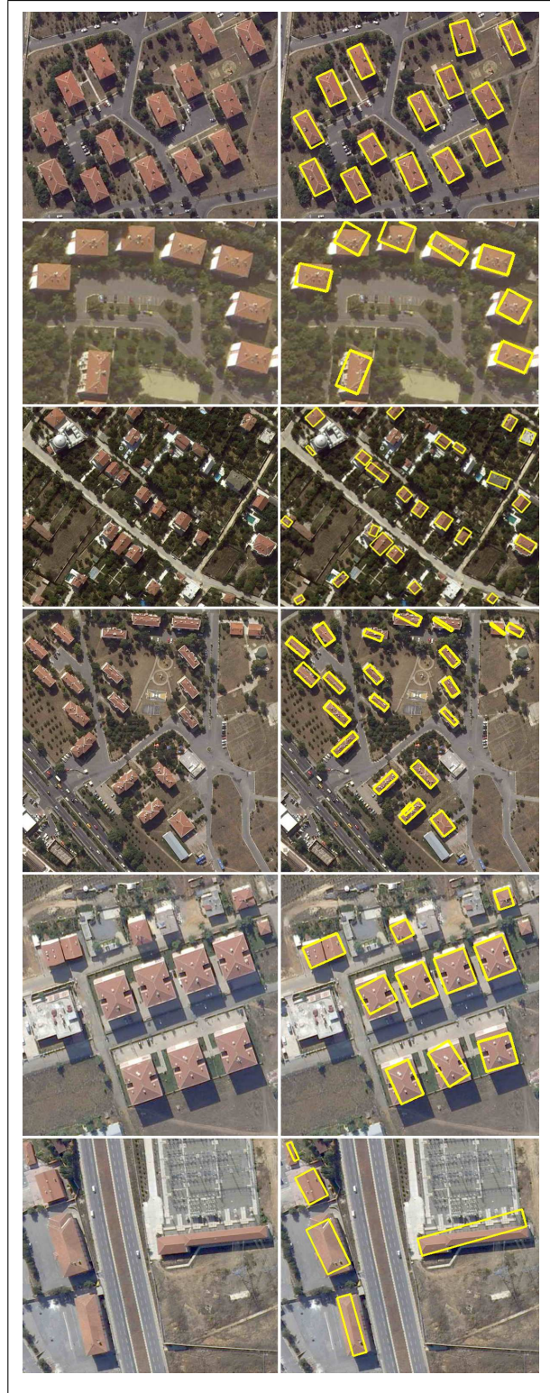
Figure 3.28. Sample building detection results using color indices in aerial images. First column: Sample test images (1,2,4,10,11,12). Second column: building detection results
