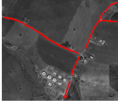
Figure 4.3. Detected road centers from the Road_1 test image by feature grouping method
