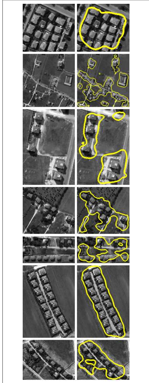
Figure 2.17. Test results with Gabor feature based algorithm for Aerial images (1 to 7) for each row separately. First column: original test images; second column: detected urban regions
