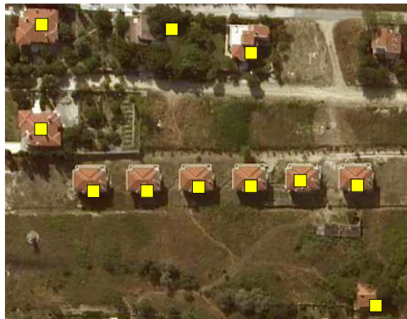
Figure 3.29. Detected buildings in Damage_1 test image. (Undamaged building measures are calculated on these detected buildings)
