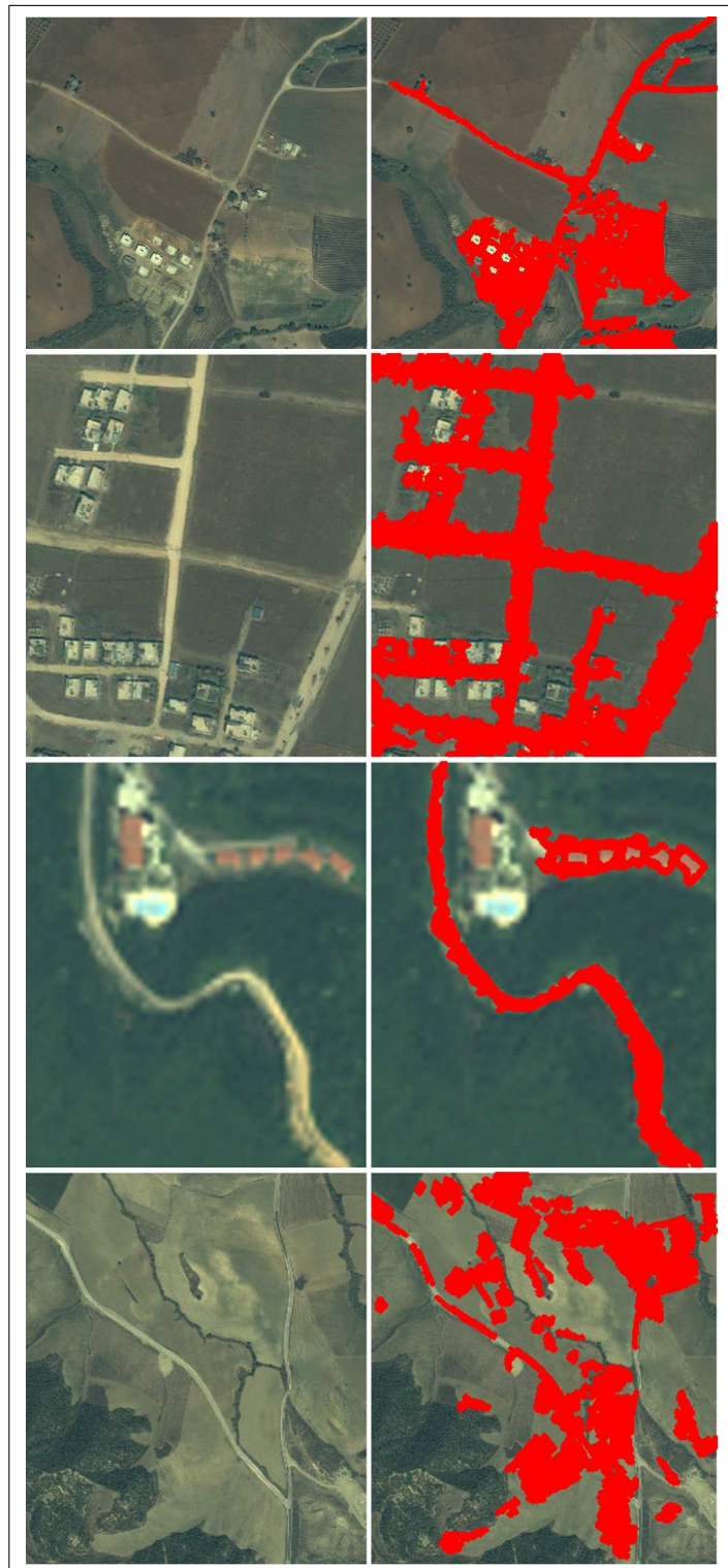
Figure 4.10. Road detection results with color feature based algorithm for color Road images (1 to 4) for each row separately. First column: original color satellite test images; second column: detected road pixels
