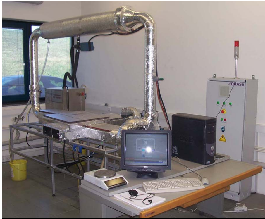
Figure 3.4. Condenser testing unit
