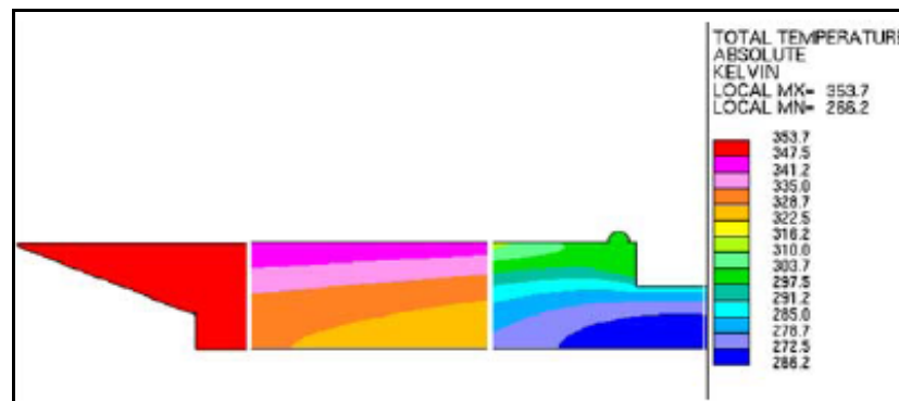
Figure 2.12. Temperature distribution of vortex tube in axial direction [61]
