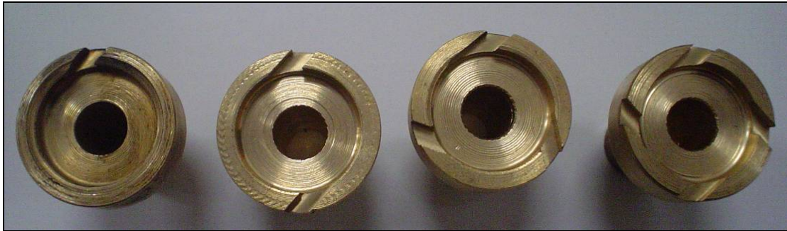
Figure 5.7. Vortex generators with inlet nozzle numbers from 1 to 4. Other geometrical parameters of the generators are all the same.
