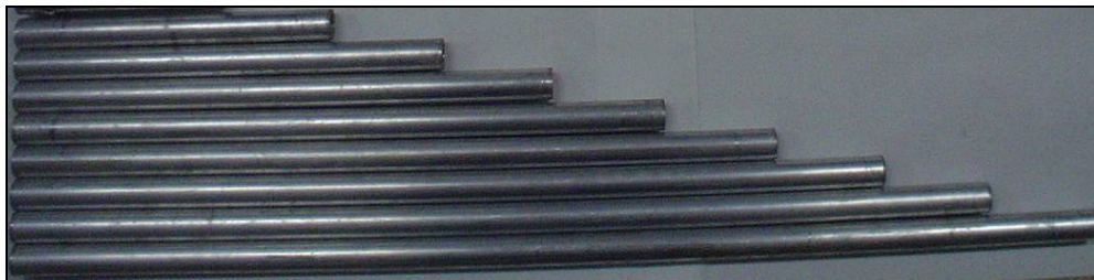
Figure 5.9. Length of the hot tubes were changed from 15D to 50D. The seamless aluminum pipes had constant diameter of 19 mm during this group of experiments.
