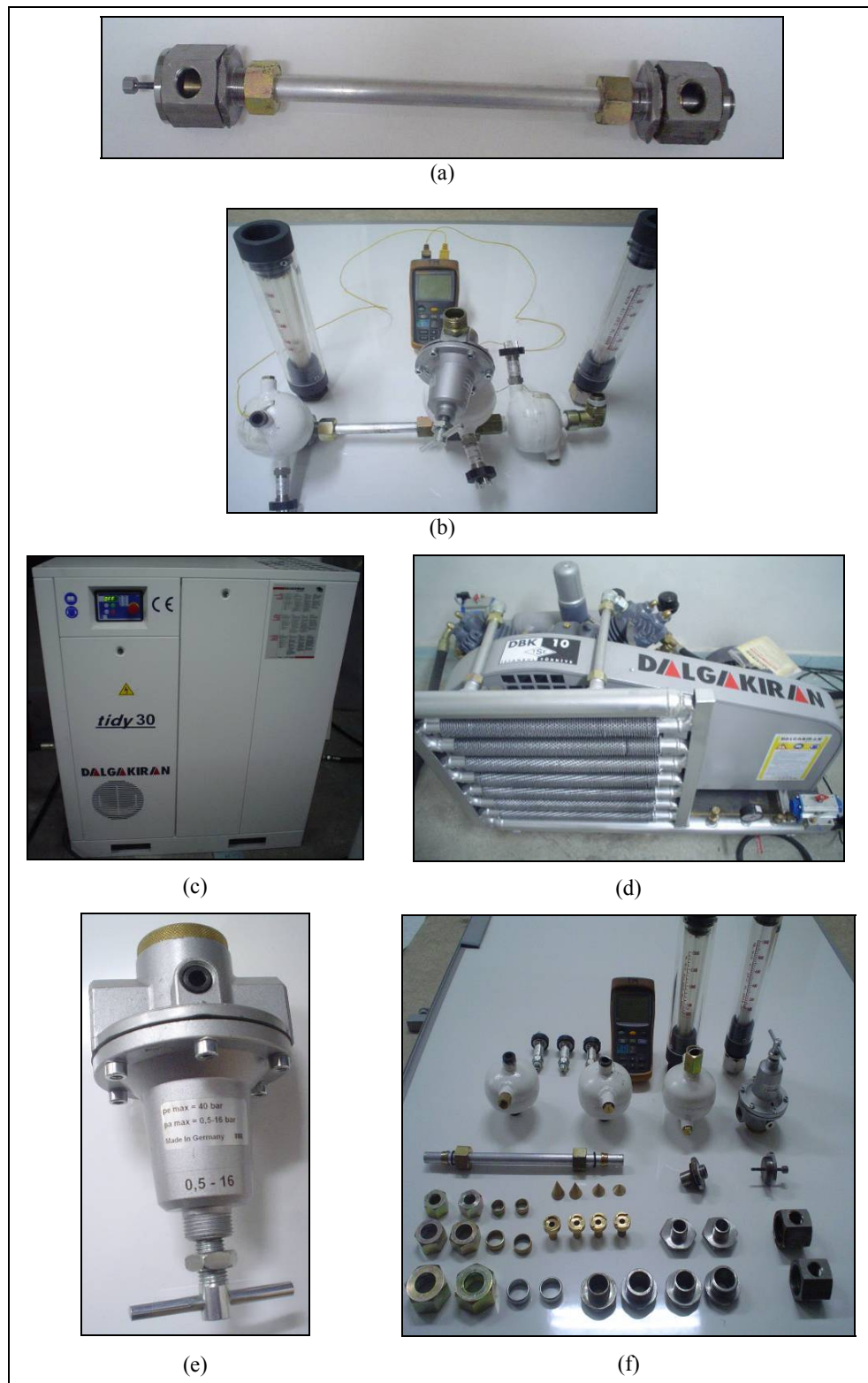
Figure 5.6. Main parts used in experiments: Vortex Tube Prototype (a), VT with installed collectors and measurement devices (b), Rotary-Screw Compressor (c), Reciprocating 'Booster' Compressor (d), pressure regulator (e) and general parts used in (f).
