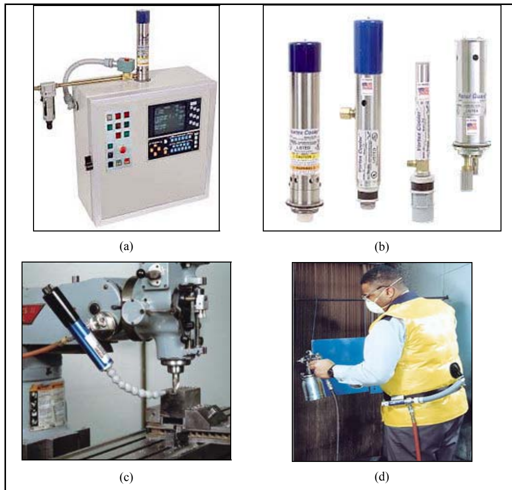
Figure 4.1. Cooling of electrical control cabinets by using commercial vortex tubes (a) and (b). In (c), spot cooling of a cutting tool in milling operation and vortex tube as a personal air-conditioner (d) [85]
