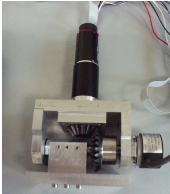
Figure 4.31 First assembled prototype of the knee joint
