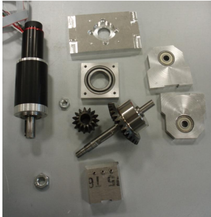
Figure 4.35 Picture of the disassembled ankle joint parts
