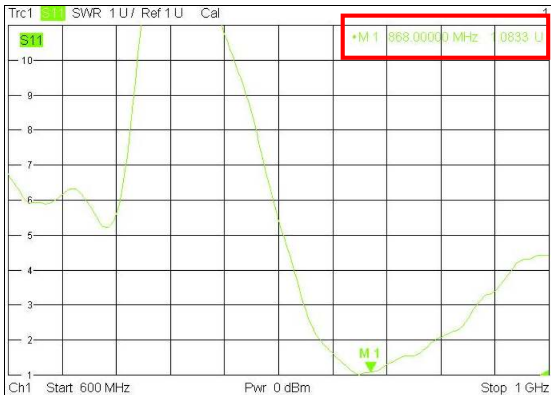
Figure 4.8. VSWR measurement for Yagi antenna
