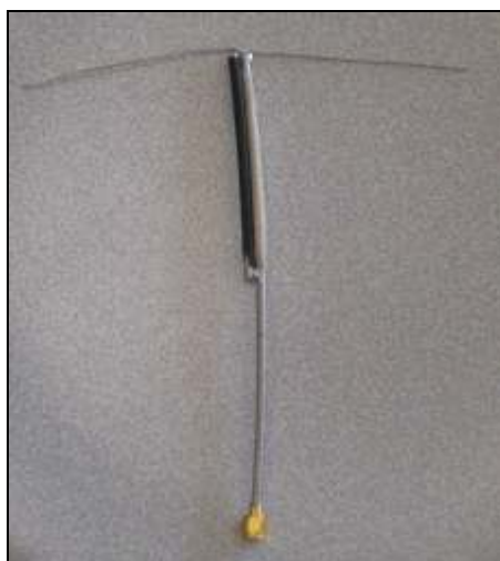
Figure 3.62. Dipole antenna with balun used during measurement as reference
