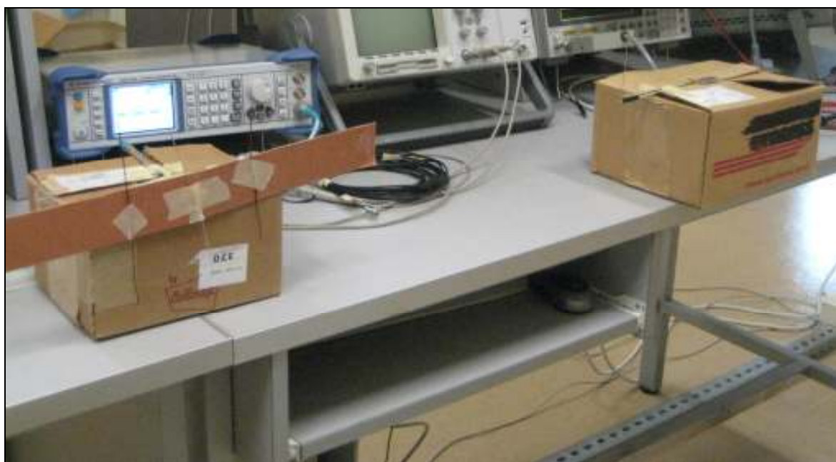
Figure 5.9. Measurement set-up when Yagi transmits and dipole antenna receives
