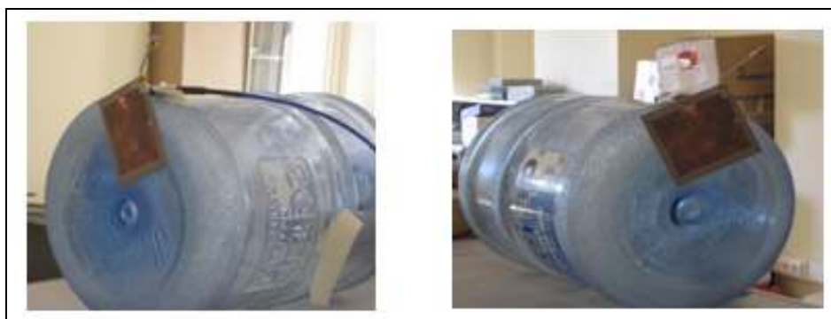
Figure 3.53. Designed tag antenna on water carboy
