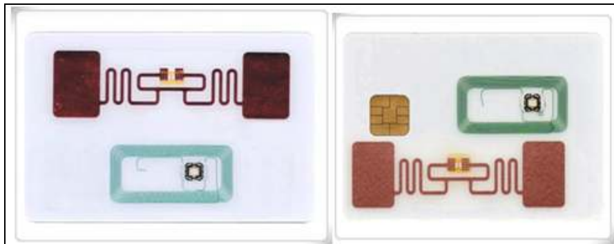
Figure 1.3. Dual band tag designed and manufactured by Cobis Corporation
