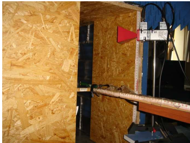
Figure 8.4. Model's measurement hole, Tx and Rx antennas
