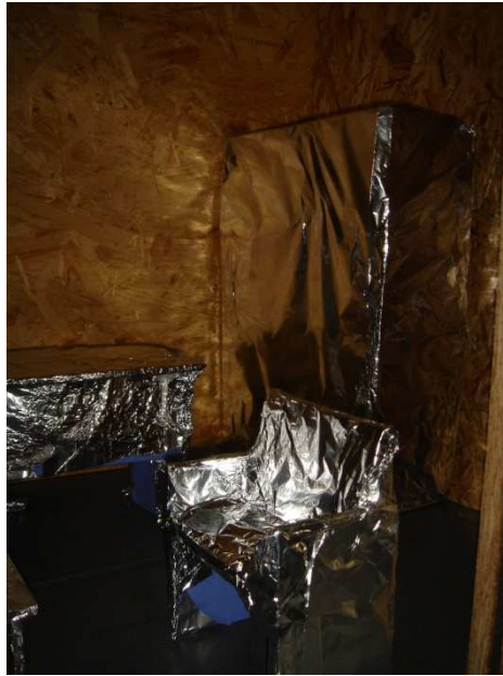
Figure 8.9. Interior side of the metallic furnished office room model (all cartoon furniture covered with aluminum foil)
