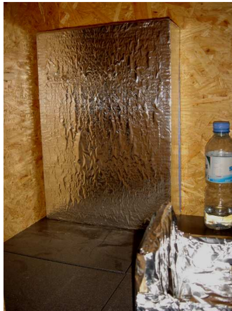
Figure 8.10. Interior side of the metallic furnished office room model (all cartoon furniture covered with aluminum foil)
