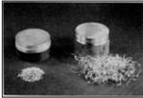
Figure 1.22. Machining chips from a P/M aluminum alloy[13]
