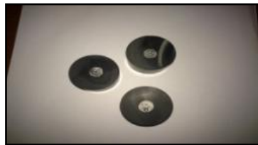
Figure 4.17. Samples in hot resin
