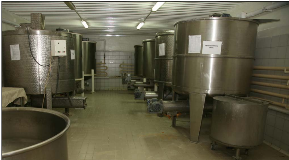
Figure B.4. Industrial tarhana fermentation (Fermentation silos and carriages)
