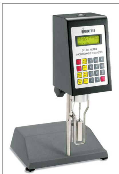
Figure 3.12. Brookfield DV-III Ultra Programmable Rheometer [78]
