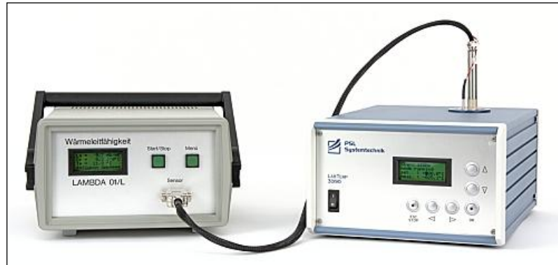
Figure 3.13. Thermal Conductivity Equipment [79]
