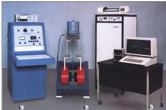
Figure 3.9. A typical Vibrating Sample Magnetometer [72]
