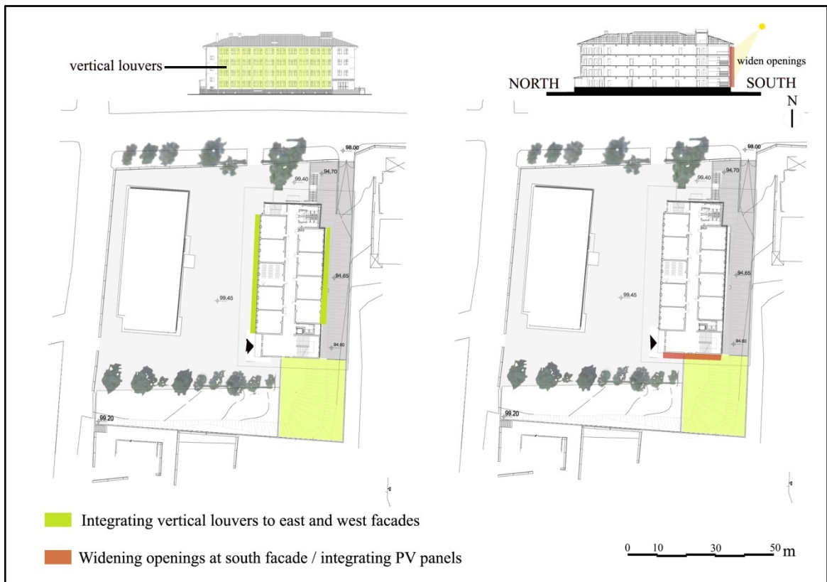
Figure 4.9. Intervention on the building envelope of the sample school building
