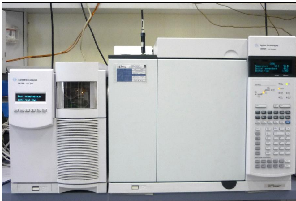
Figure 4.6. Agilent 7890 gas chromatograph and divinylbenzene-carboxen-polydimethylsiloxane coated fiber injected to the port
