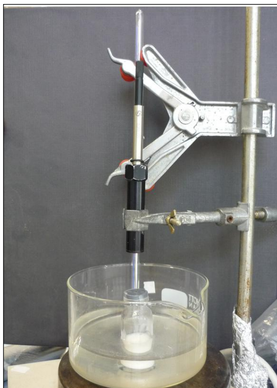
Figure 4.5. Transaction of divinylbenzene-carboxen-polydimethylsiloxane-coated fiber with the headspace of milk sample
