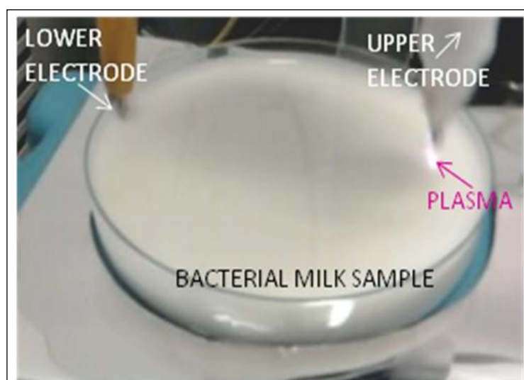
Figure 4.2. Plasma discharge occurring on the milk surface by high voltage (9 kV) applied between upper (on the right) and lower electrodes (on the left)
