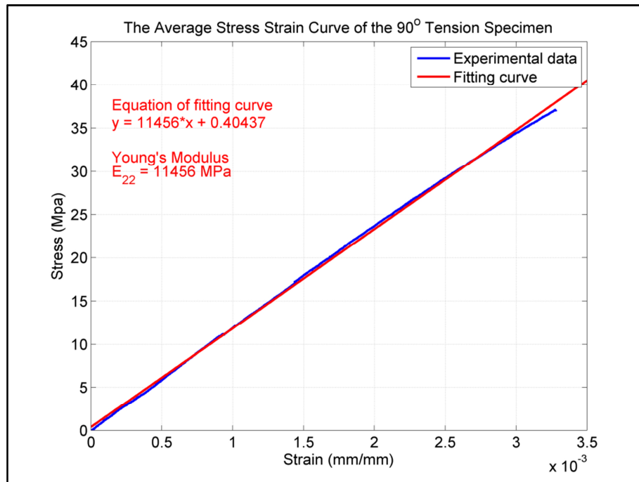
Figure 3.6. The average stress-strain curve of the 90° specimen UDT1
