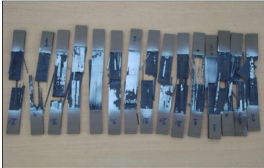
Figure 3.23. Tested coupons after failure during the fatigue test
