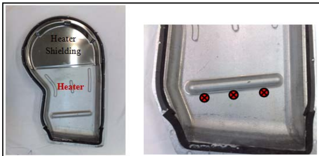
Figure 3.15. Relative humidity sensor location at the drum inlet
