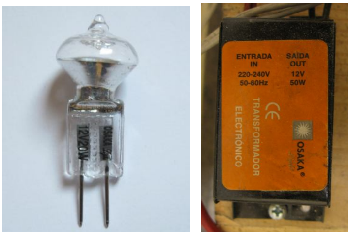
Figure 7.4. The lamp and electronic transformer used in the experiments related to GaInSn alloy (Halogen lamp 12V, 20W, Osaka Light)
