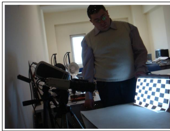
Figure 3.5. An example on image taking for calibration
