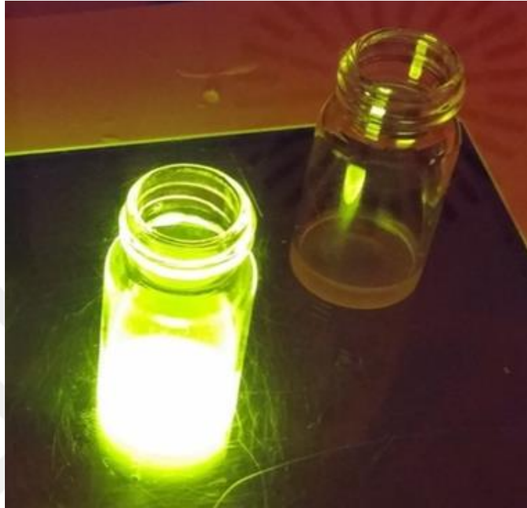
Figure 2.12.: Fluorescence intensity difference between induced and un-induced YFP-R5 under blue light illumination. YFP-R5 in this image is concentrated after purification by a ratio of 5.
