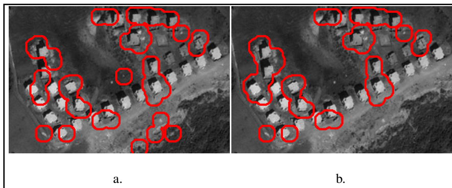
Figure 5.13. Graph matching based comparison results: a. Using only spatial constraints; b. Adding three neighborhood constraint
