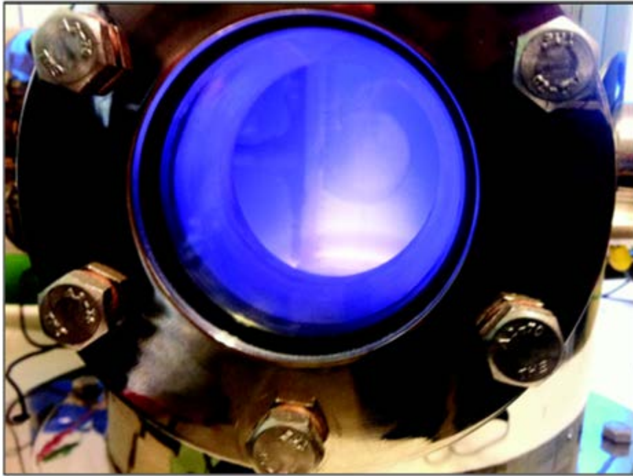
Figure 5.5. The view of the glow discharge probe measurements at the outside of the chamber
