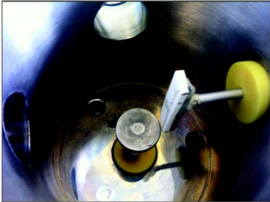
Figure 5.7. Inside of the vacuum chamber with probes
