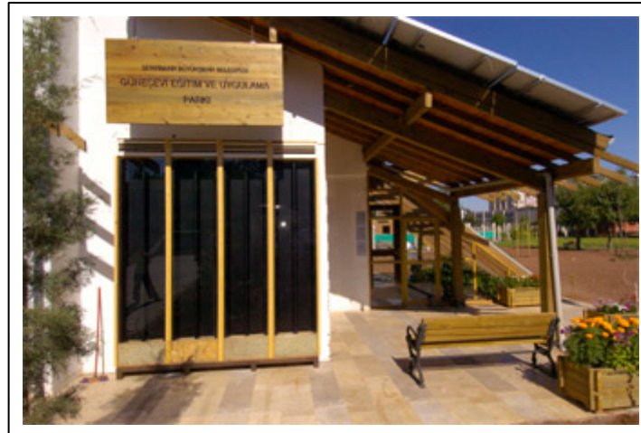
Figure 4.20. Trombe walls of Diyarbakır solar house [46]
