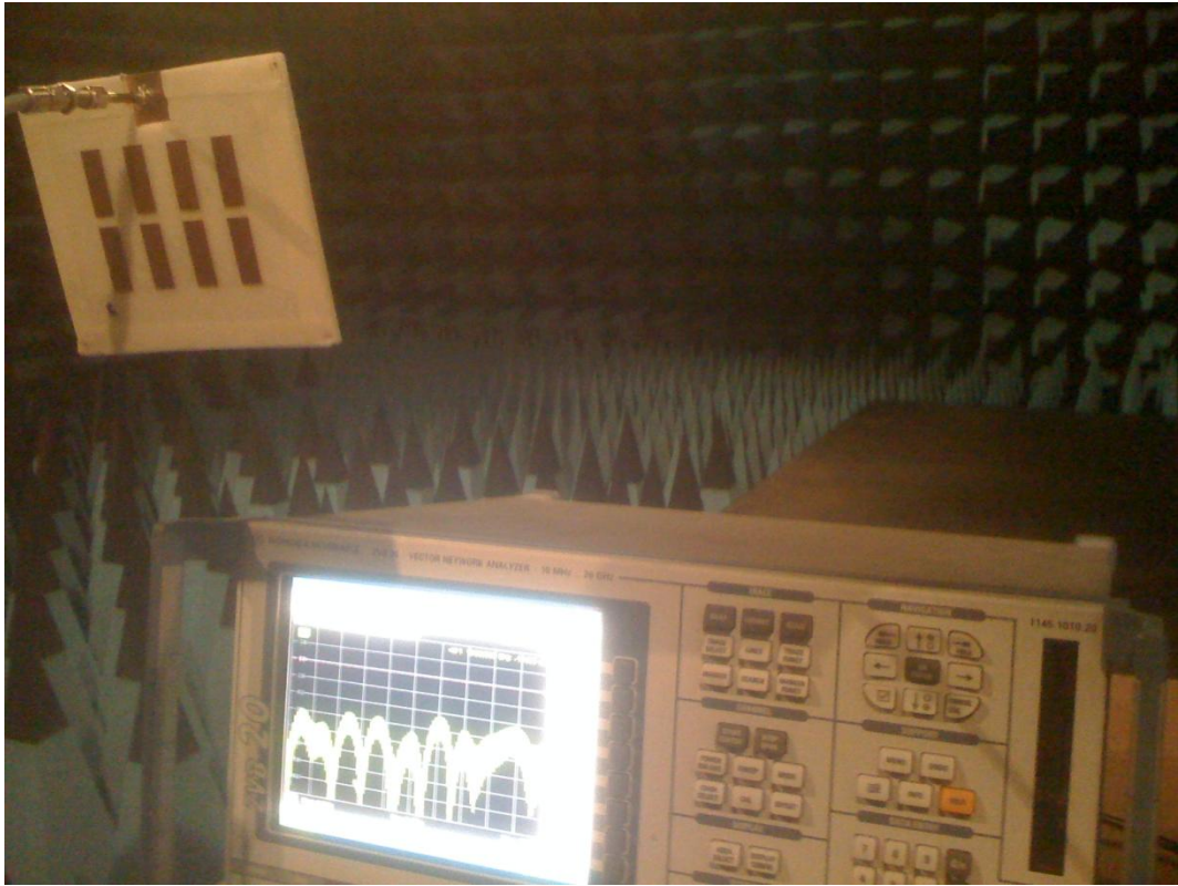
Figure 2.78. Measurement Set up in Anechoic Chamber
