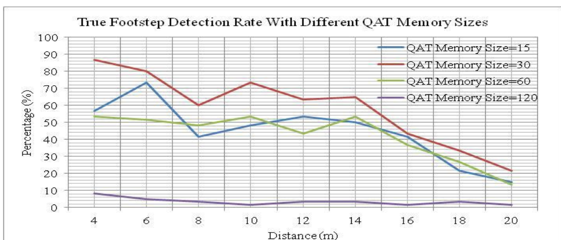
Figure 7.17. True footstep detection rate with different QAT memory sizes (Person B)
