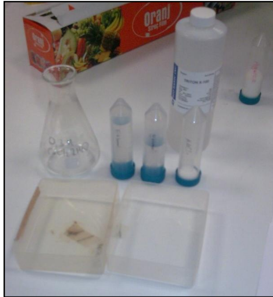
Figure 3.5. The materials and quantities for tumor phantom construction
