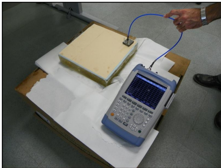
Figure 3.1. Experimental setup of the microwave imaging system
